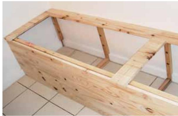
**6** Strengthen the seat flaps (A x 2) with three supports (B x 3) each on the underside as shown, since these will take the full weight of any load and may bow or break after continued usage. Install the reinforced seat flaps (A x 2, B x 6) using piano hinge along the adjoining edges at the back. Take care to align the sections accurately and with equal spacing since this will be visible from the exterior.
